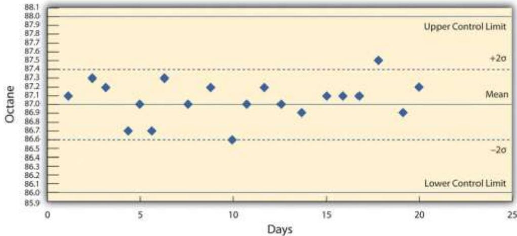
She recognizes that the highest and lowest measurements are not part of a trend and are probably due to chance causes. However, the control chart from the next twenty days, as shown below, indicates an upward trend that might be due to an assignable cause. She alerts the process manager to let him know that there is a problem that needs to be fixed before the product exceeds the upper control limit. This might indicate the need to initiate a project to fix the problem.
