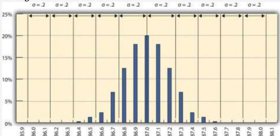
The refinery's quality control manager calculates that the new standard deviation is 0.2 octane. From this, he can use the 68-95-99.7 rule to estimate that 68.3 percent of the fuel produced will be between sigma 86.8 and 87.2 and that 99.7 percent will be between 86.4 and 87.6 octane. A shorthand way of describing this amount of control is to say that it is a five-sigma production system, which refers to the five standard deviations between the mean and the control limit on each side.
