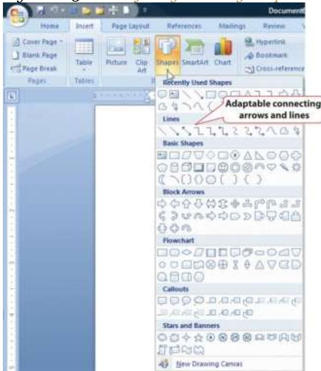
Adaptable connecting lines and arrows can be used that redraw automatically when the shapes are moved. This feature facilitates rapid revisions when the shapes must be moved, because the connecting arrows do not need to be redrawn.
